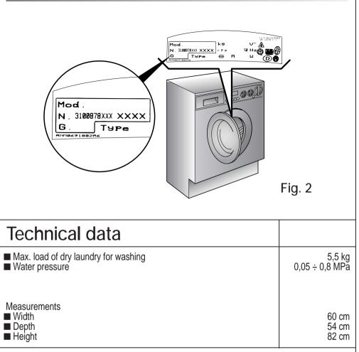
NB: For specifications regarding electrical data, see the data panel on the front of the washing machine (porthole area) - as shown in diagram above.
